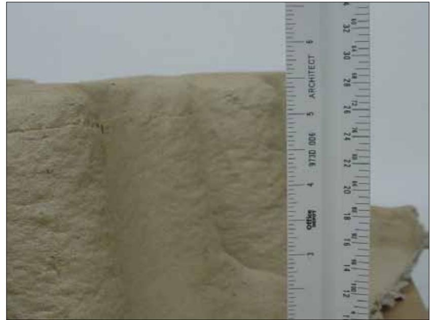
**Molded Pulp Former - 5 ½” Thick Concrete Capacity**
